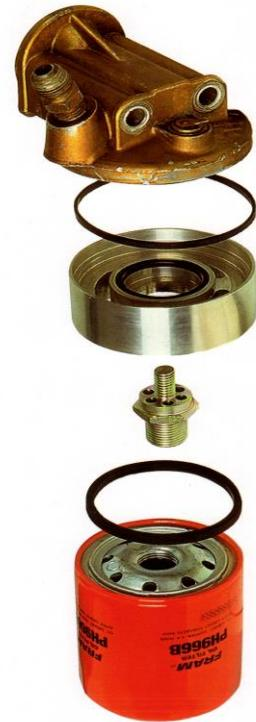
Remove the old oil filter and can. Remove the old rubber sealing ring which is probably jammed into the groove in the alloy filter housing on the engine. (You are advised to wait until the old oil has stopped dripping out.) It's not unknown for there to be two old seals jammed into the groove, which explains why so many filter housings leak. Clean the housing, removing any old gasket cement etc. Remove the splash plate (looks like a big flat washer) and snap ring.
